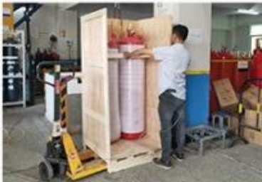
Reinforced wooden frame
